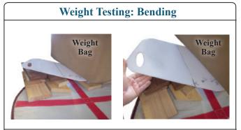
When the weight was left for several minutes half way across the gap, the 6mm Slide Board developed a bend that was big enough to put some fingers under. When the weight was removed the Slide Board straightened out again.
